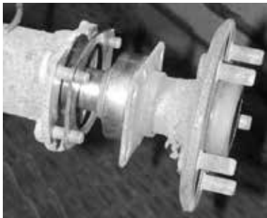
Installation of Spacer Plate.
