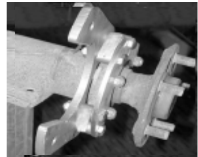
Installation of caliper bracket.
