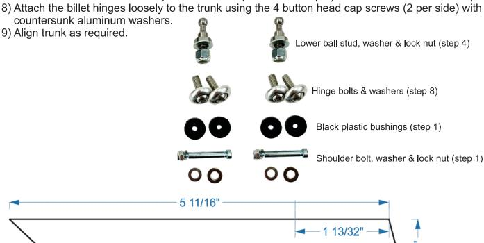
Driver Side - flip for passenger side Verify template measurements after printing.
